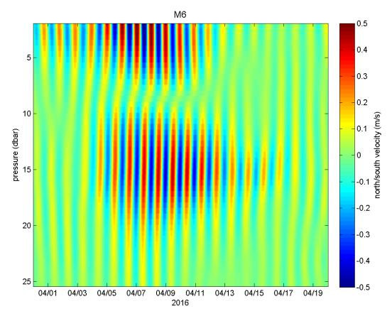
Near-inertial velocities are strong and show the classic two-layer form with opposing phases above and below the pycnocline. As shown by Simpson et al. (2002) and others, for a coastal environment, energy does not have to transfer through the pycnocline to drive the lower layer oscillations, but can be driven instead by sea-surface setup/set-downs against the coast.
