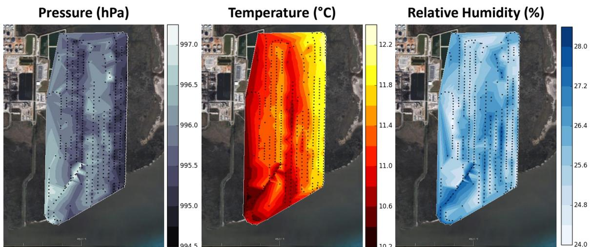
**Figure 4. UAS-measured pressure, temperature, and relative humidity at 225m AGL altitude over the November 23, 2015 test flight over Grand Bay NERR test flight. Black points represent UAS observation locations.**
