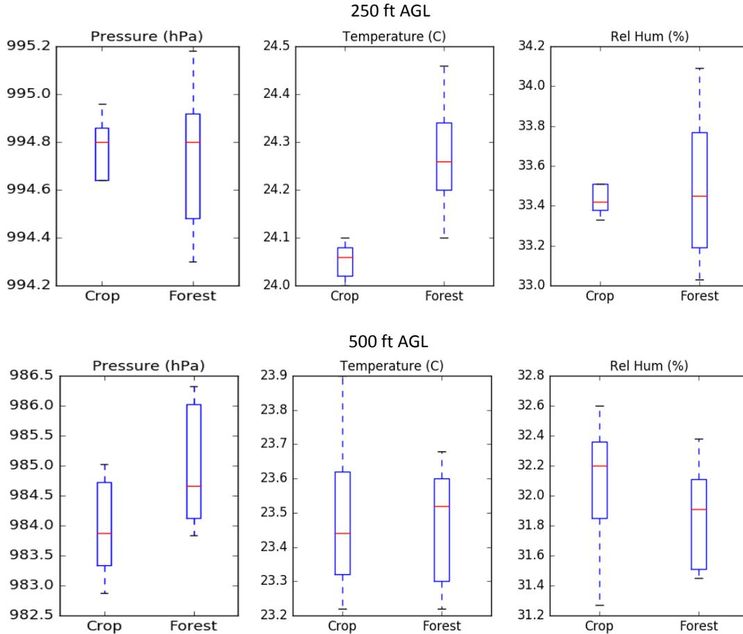
**Figure 6. Box and whisker plots of bootstrap resampled meteorological data over crop and forest land covers measured at 250 ft and 500 ft AGL UAS flights over MSU research farm. The median of each plot is denoted by the horizontal red line, the limits of the box are the 25<sup>th</sup>/75<sup>th</sup> percentiles, and the whiskers denote the 5<sup>th</sup>/95<sup>th</sup> percentiles.**
