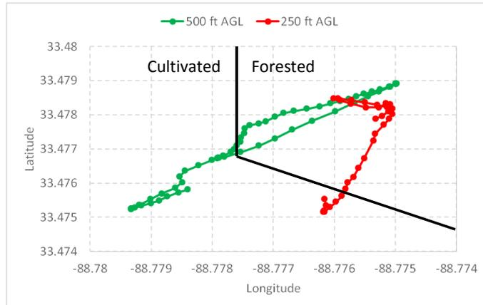
**Figure 5. Observation points associated with 250 ft (red) and 500 ft (green) AGL flight paths, conducted on April 22, 2016 at MSU research farm. The colors correspond to the flight paths shown in Fig. 2. Black lines denote approximate boundary of cultivated-forested land cover boundary.**
