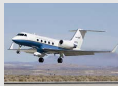
NASA's G-III research aircraft carrying the pod-mounted synthetic aperture radar on takeoff. (NASA photo)
