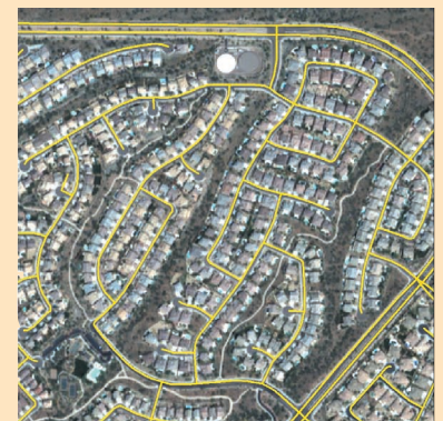
Figure 3. High-resolution panchromatic (upper left), color (upper right) or color infrared (left) images from DigitalGlobe's QuickBird satellite may be used as a backdrop for screen digitizing. Such sources of accurate image data are used as a base layer for aligning road centerline data sets.
