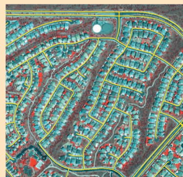
Figure 3. High-resolution panchromatic (upper left), color (upper right) or color infrared (left) images from DigitalGlobe's QuickBird satellite may be used as a backdrop for screen digitizing. Such sources of accurate image data are used as a base layer for aligning road centerline data sets.
