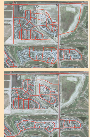
Figure 2. The MTAIP aims to improve the accuracy on the U.S. Census Bureau TIGER file by collecting accurate data from state, county, local and tribal agencies that have used highly accurate image data to realign centerline data sets.
