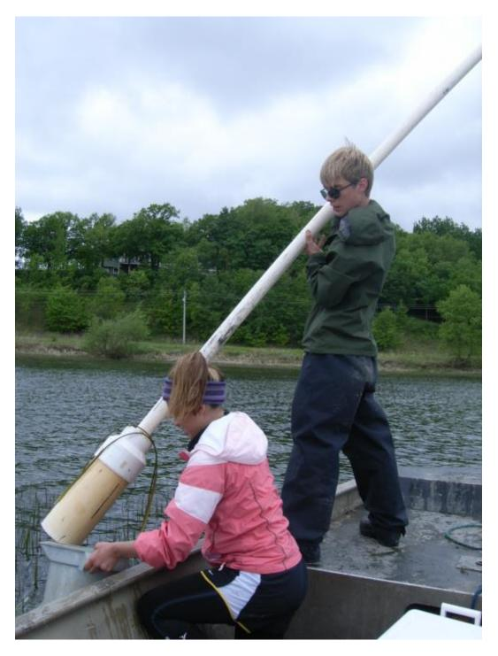
Figure 5. The 6" diameter-coring device used to collect aboveground and belowground biomass of flowering rush in the Detroit Lakes.
