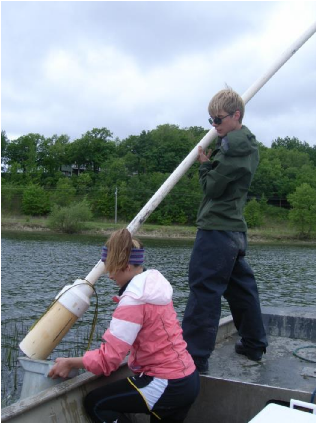
Figure 5. The 6" diameter coring device used to collect aboveground and belowground biomass of flowering rush in the Detroit Lakes.
