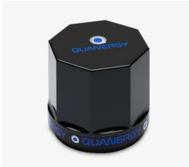
Figure 13: Quanergy M8-1 LIDAR
