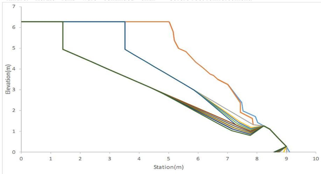
Graph 1 Streambank 6 left side geometry for, flow depth=3m, tension crack=1.5m after failure occur.
