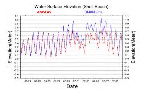
FIG. 20. Observed water level (blue) and predicted water AMSEAS water level (red) for Shell Beach CMAN station in Lake Borgne, LA, during 0000 UTC 15 June to 0000 UTC 15 July 2010 relative to NAVD88. Above average water elevation associated with Hurricane Alex and the non-tropical low pressure system are apparent on 29 June-1 July and 3-7 July, respectively.
