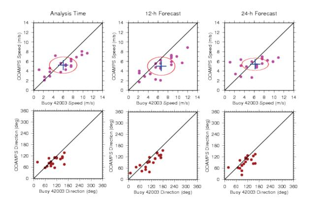
FIG. 6. Example of scatterplots for COAMPS wind initialization as well as 12- and 24-hr forecasts for speed (upper) and direction (lower) interpolated to buoy 42003 during the same period as Fig. 5. Wind speed plots also include ovals representing one standard deviation of each dataset; circular plots indicate both the model and buoys have the same data ranges and elliptic plots indicate one dataset has less range than the other.
