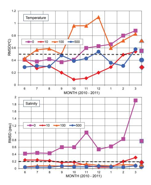
FIG. 23. Month-by-month mean temperature (upper) and salinity (lower) root mean square differences (RMSD) at the surface, 10-, 100-, and 500-m depths. Dashed lines represent tolerance goals of  $\pm 0.5^{\circ}$ C for temperature and  $\pm 0.20$  psu for salinity. The 10-month (June 2010 – March 2011) means at the right are reflected in Column 10 of Table V.
