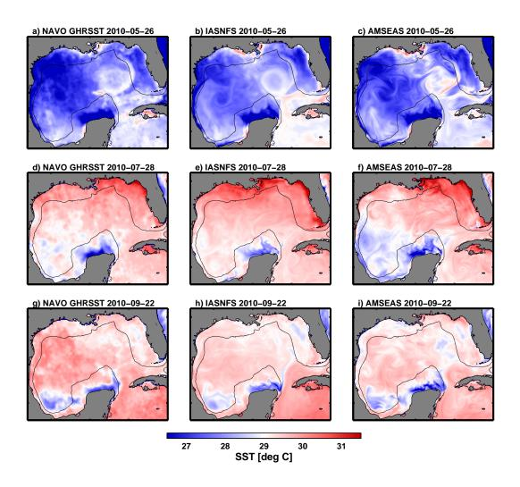
FIG. 3. Comparison of sea-surface temperature (SST) in NAVO GHRSST analysis (a, d, g – derived from multiple satellite measurements), IASNFS nowcast (b, e, h), and AMSEAS nowcast (c, f, i), for three dates in 2010. The solid contour represents the 500-m isobath.
