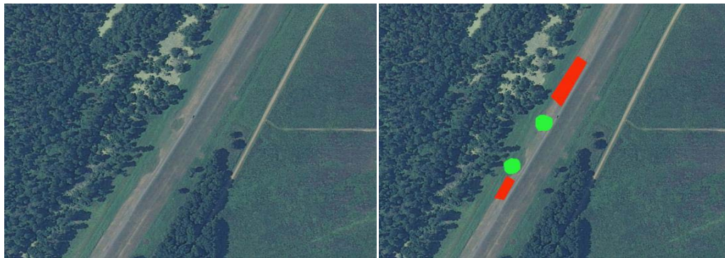
Figure 1. Left Image: Actual levee segment. Right Image: Mask segment. Green: landslide; Red: healthy levee.
