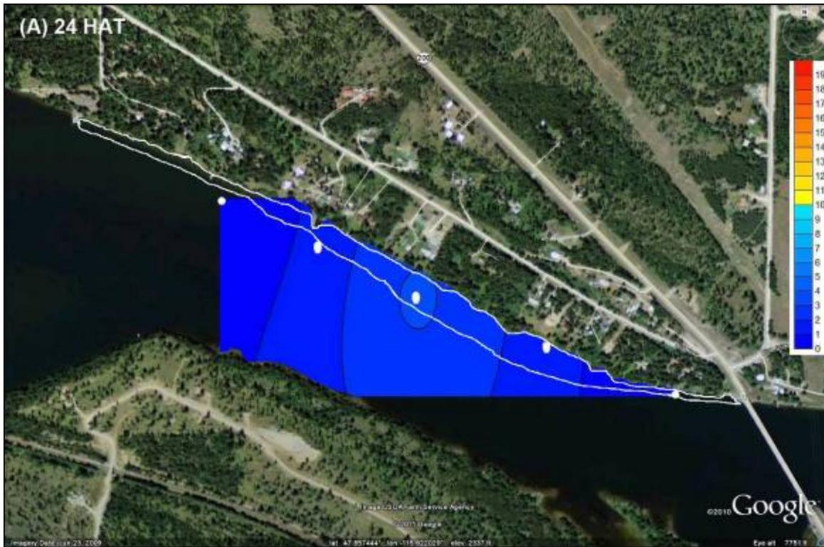
Figure 2.27. Predicted rhodamine dye dissipation from the bottom of the water column from plot 8 at 24 HAT (A) according to the Kriging interpolation method from 5 water sampling stations, July 2010.
