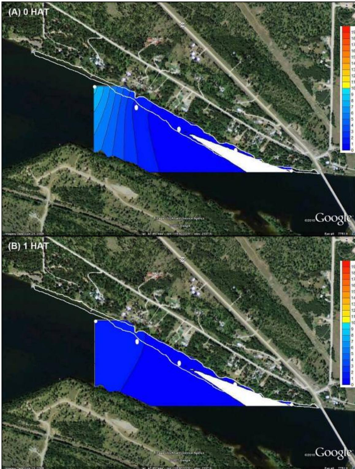
Figure 2.21. Predicted rhodamine dye dissipation from the middle of the water column from plot 8 at 0 HAT (A) and 1 HAT (B) according to the Kriging interpolation method from 5 water sampling stations, July 2010.
