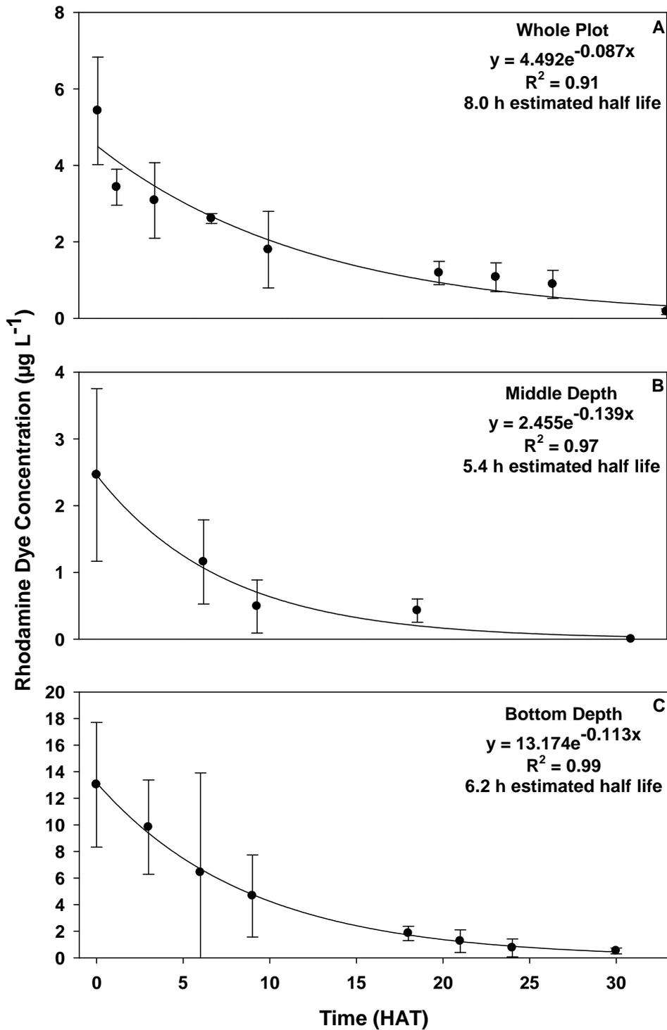
Figure 2.5. Rhodamine dye concentrations and respective half lives for the whole plot (A), middle depth (B), and bottom depth (C) for plot 7 (triclopyr alone) in Noxon Rapids Reservoir, July 2010.
