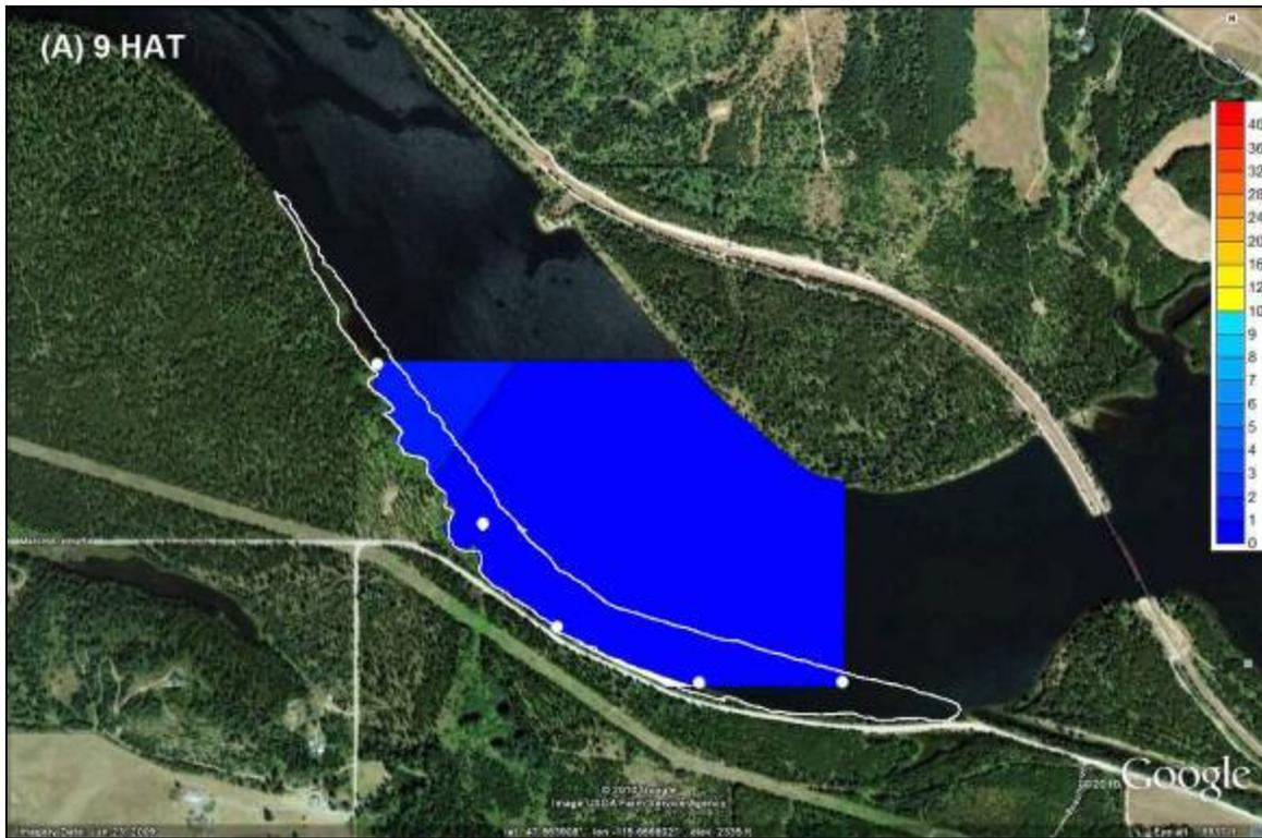
Figure 2.11. Predicted rhodamine dye dissipation from the middle of the water column from plot 7 at 9 HAT according to the Kriging interpolation method from 5 water sampling stations, July 2010.
