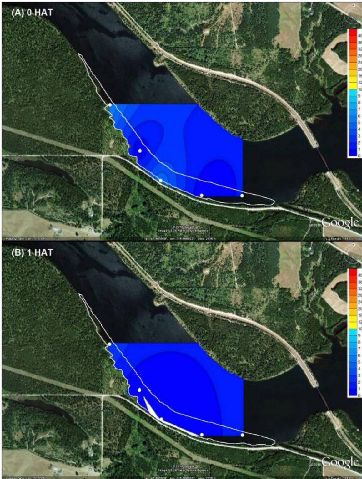
Figure 2.9. Predicted rhodamine dye dissipation from the middle of the water column from plot 7 at 0 HAT (A) and 1 HAT (B) according to the Kriging interpolation method from 5 water sampling stations, July 2010.
