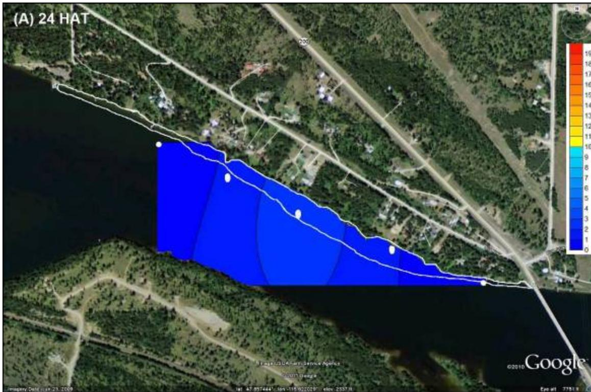
Figure 2.23. Predicted rhodamine dye dissipation from the middle of the water column from plot 8 at 24 HAT (A) according to the Kriging interpolation method from 5 water sampling stations, July 2010.
