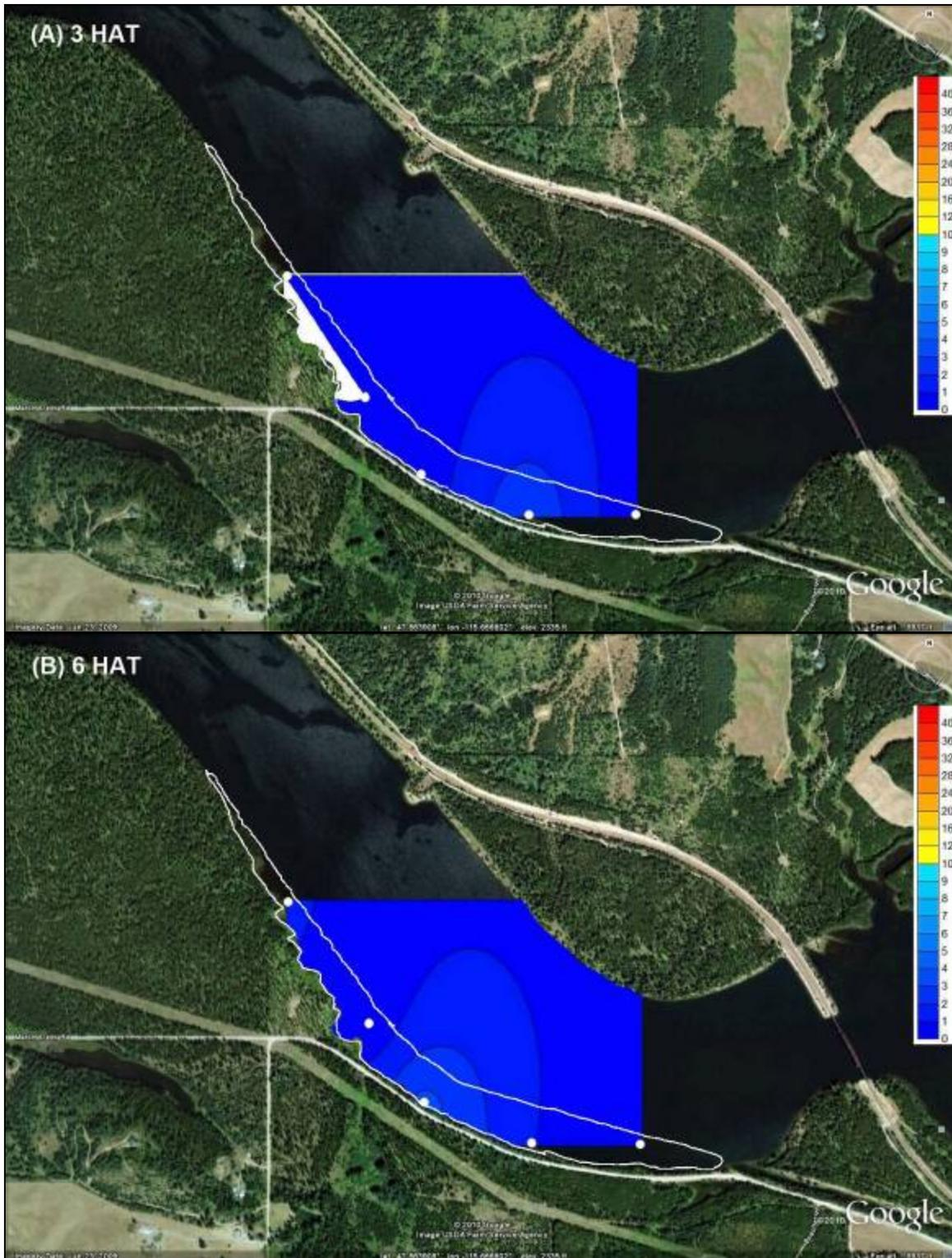
Figure 2.10. Predicted rhodamine dye dissipation from the middle of the water column from plot 7 at 3 HAT (A) and 6 HAT (B) according to the Kriging interpolation method from 5 water sampling stations, July 2010.
