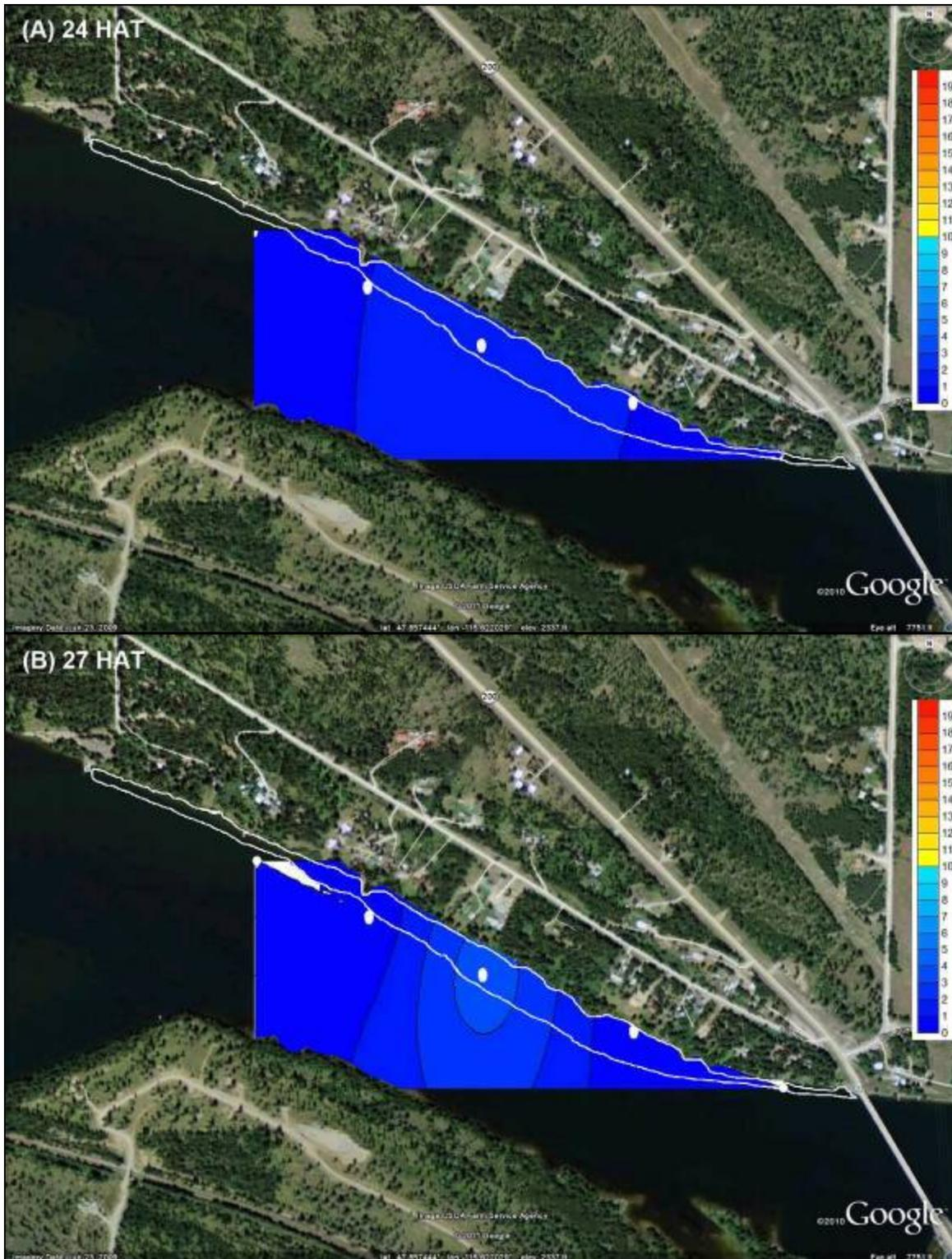
Figure 2.20. Predicted rhodamine dye dissipation from the top of the water column from plot 8 at 24 HAT (A) and 27 HAT (B) according to the Kriging interpolation method from 5 water sampling stations, July 2010.
