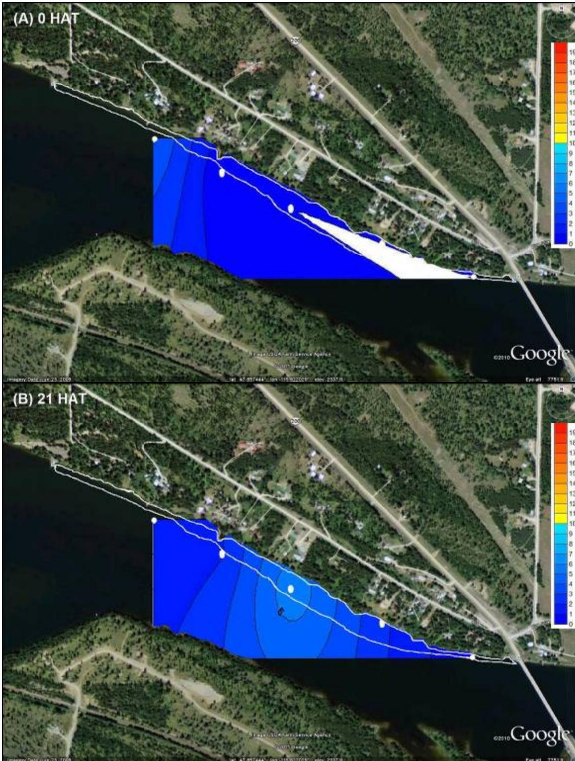
Figure 2.19. Predicted rhodamine dye dissipation from the top of the water column from plot 8 at 0 HAT (A) and 21 HAT (B) according to the Kriging interpolation method from 5 water sampling stations, July 2010.
