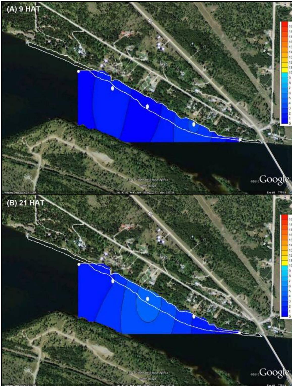
Figure 2.22. Predicted rhodamine dye dissipation from the middle of the water column from plot 8 at 9 HAT (A) and 21 HAT (B) according to the Kriging interpolation method from 5 water sampling stations, July 2010.
