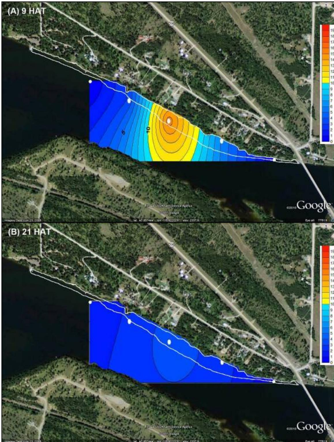
Figure 2.26. Predicted rhodamine dye dissipation from the bottom of the water column from plot 8 at 9 HAT (A) and 21 HAT (B) according to the Kriging interpolation method from 5 water sampling stations, July 2010.
