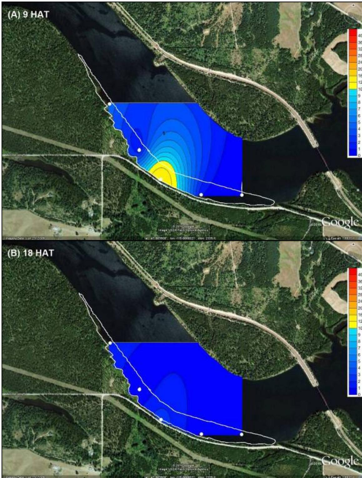
Figure 2.14. Predicted rhodamine dye dissipation from the bottom of the water column from plot 7 at 9 HAT (A) and 18 HAT (B) according to the Kriging interpolation method from 5 water sampling stations, July 2010.
