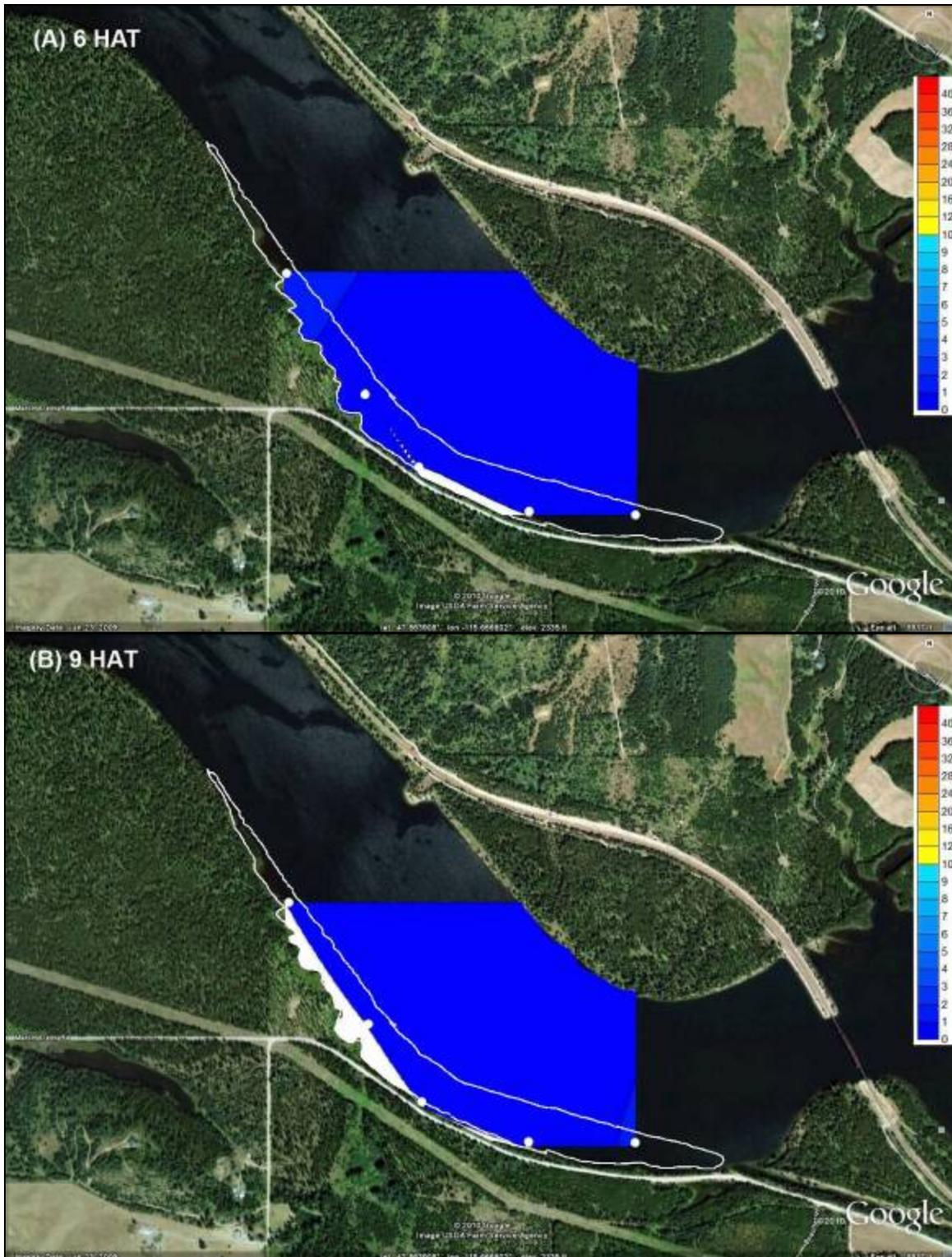
Figure 2.7. Predicted rhodamine dye dissipation from the top of the water column from plot 7 at 6 HAT (A) and 9 HAT (B) according to the Kriging interpolation method from 5 water sampling stations, July 2010.
