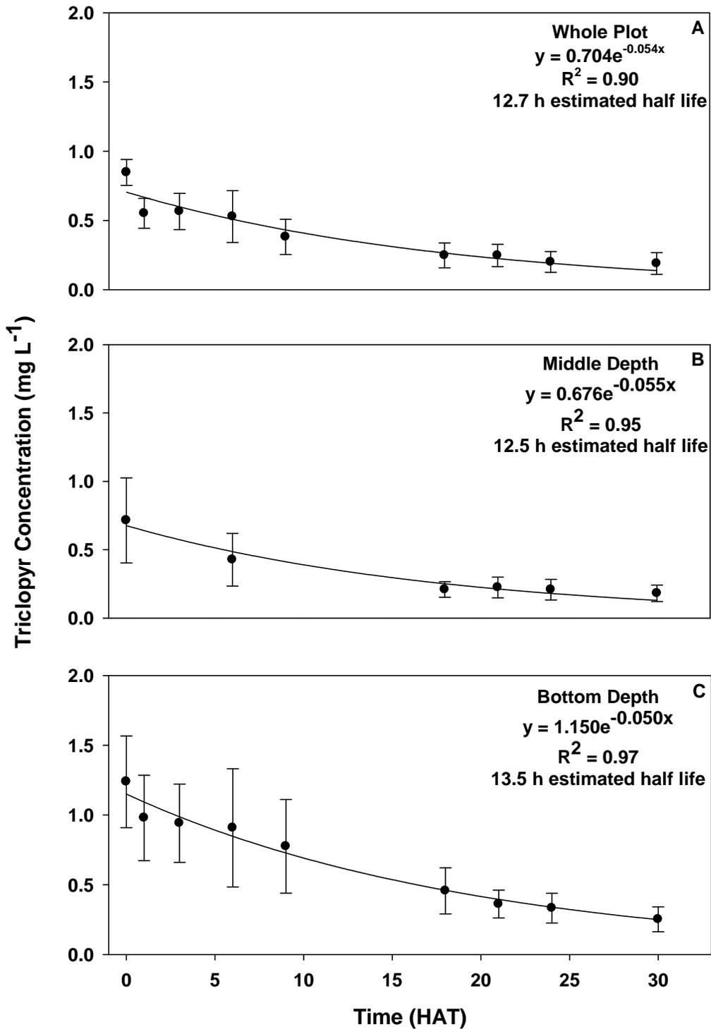
Figure 2.16. Triclopyr concentrations and respective half lives for the whole plot (A), middle depth (B), and bottom depth (C) for plot 7 (triclopyr alone) in Noxon Rapids Reservoir, July 2010.
