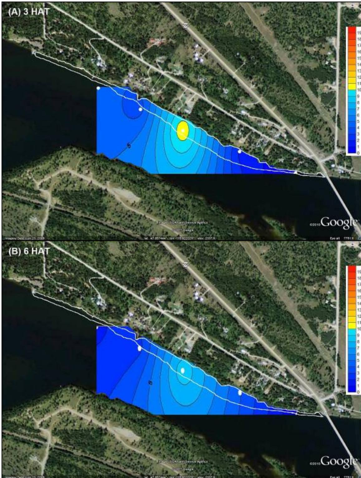
Figure 2.25. Predicted rhodamine dye dissipation from the bottom of the water column from plot 8 at 3 HAT (A) and 6 HAT (B) according to the Kriging interpolation method from 5 water sampling stations, July 2010.
