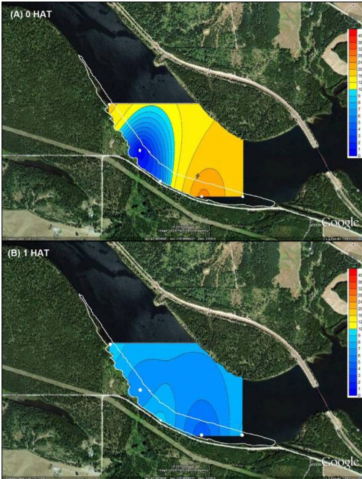
Figure 2.12. Predicted rhodamine dye dissipation from the bottom of the water column from plot 7 at 0 HAT (A) and 1 HAT (B) according to the Kriging interpolation method from 5 water sampling stations, July 2010.
