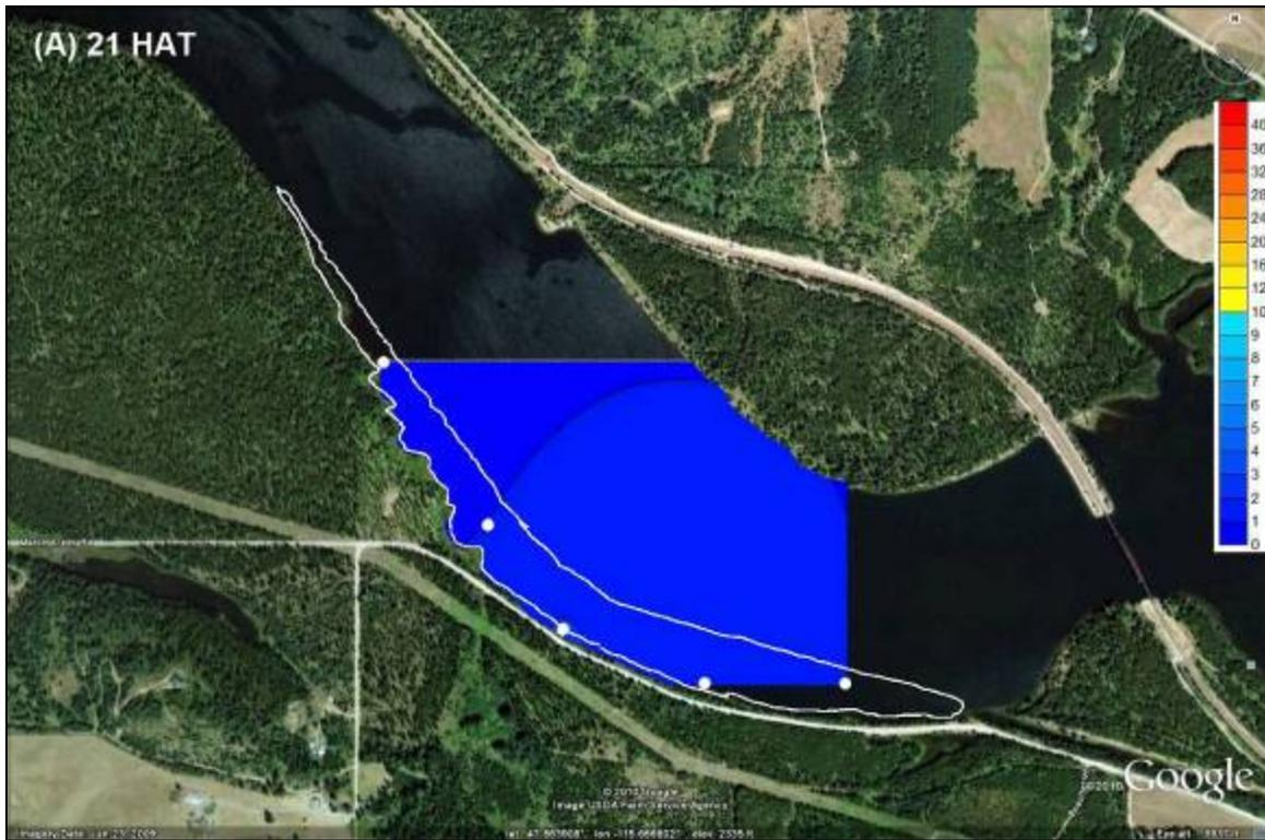
Figure 2.8. Predicted rhodamine dye dissipation from the top of the water column from plot 7 at 21 HAT (A) according to the Kriging interpolation method from 5 water sampling stations, July 2010.
