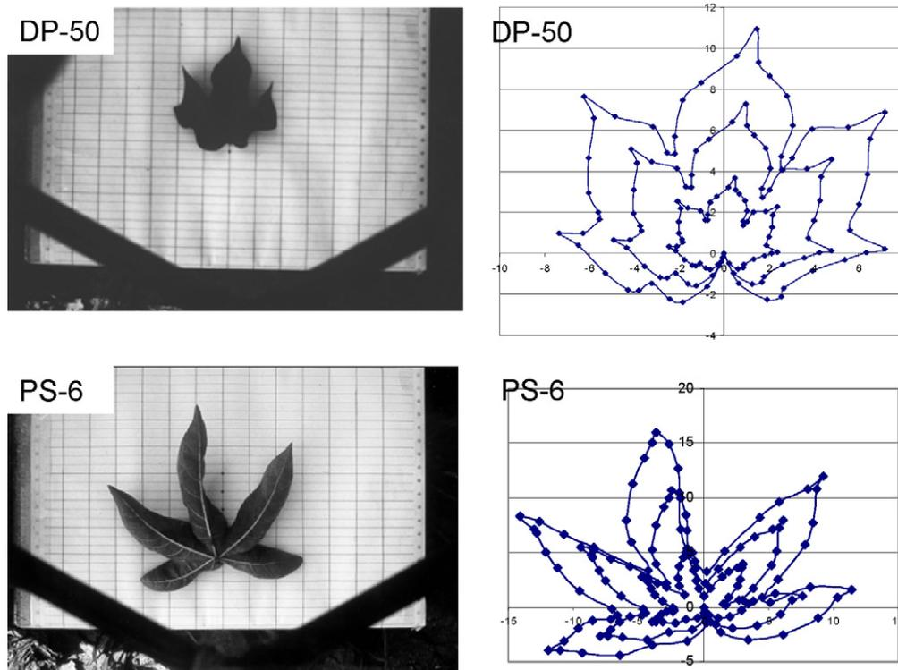
**Fig. 4.** Individual leaves were photographed over a gridded plate to obtain detailed information on individual leaf geometry. Close-range photogrammetry techniques were used for estimating  $(X, Y, Z)$  coordinates of several points over the surface of the leaves (benchmark points). Those coordinates were used for interpolating individual leaf surfaces (through CAGD) for each of the cotton cultivars included in this study.
