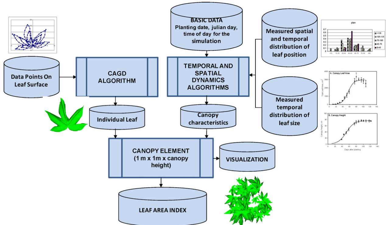
**Fig. 6.** Flow chart of model development. Points measured on the leaf surface are used to generate a geometrical model of an individual leaf through the CAGD algorithm. Measured temporal and spatial algorithms of leaf position and size are used to place the individual leaves into a canopy element of  $1 \text{ m} \times 1 \text{ m} \times \text{canopy-height}$ .
