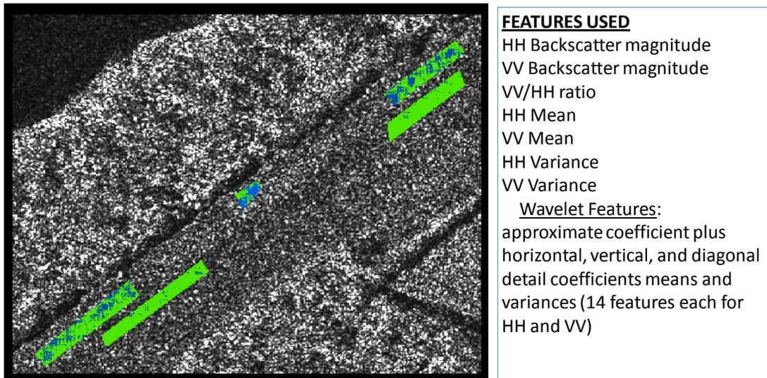
Figure 4: Illustrating the SAR imagery from the levee area, the classification results and test areas (blue: detected landslide, green: test area masks), and the features used for this classification task. The overall accuracy for this particular experiment was 67%.
