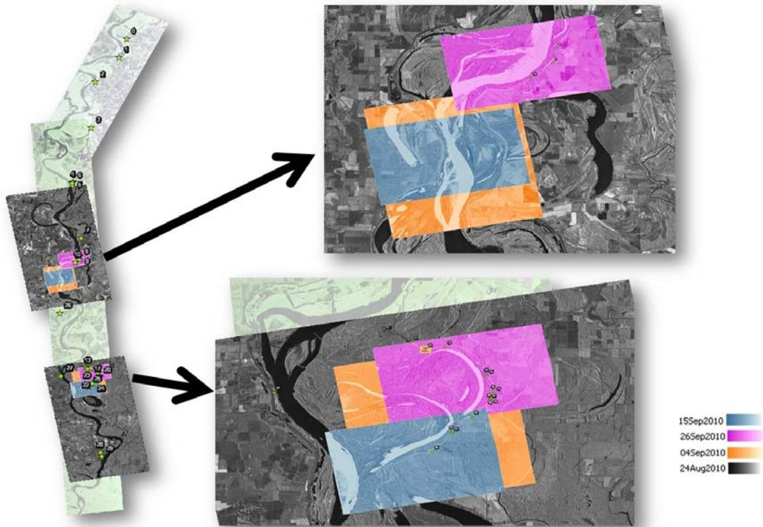
Figure 2: TerraSAR-X radar backscatter in both HH and VV polarizations were acquired on four successive cycles in 2010. The overall project study area covers 130 km of the Mississippi river valley along the western border of the state of Mississippi.
