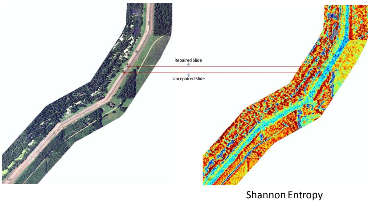
Figure 3: Illustrating the Shannon Entropy feature over a section of the Mississippi Levee system. High spatial resolution optical image (left) and Shannon Entropy (right). Notice the slides (repaired and unrepaired) show up as anomalies when visualizing the entropy feature within the levee area.
