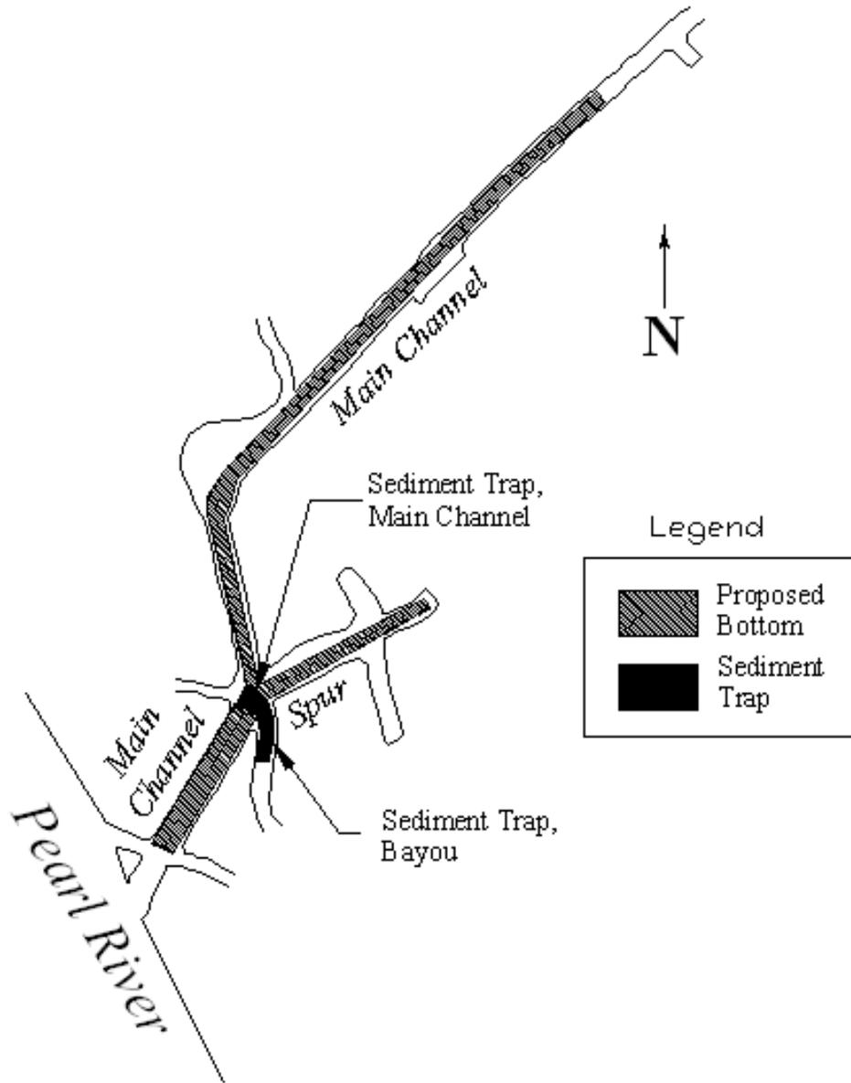
Figure 29 Sediment Trap Location
