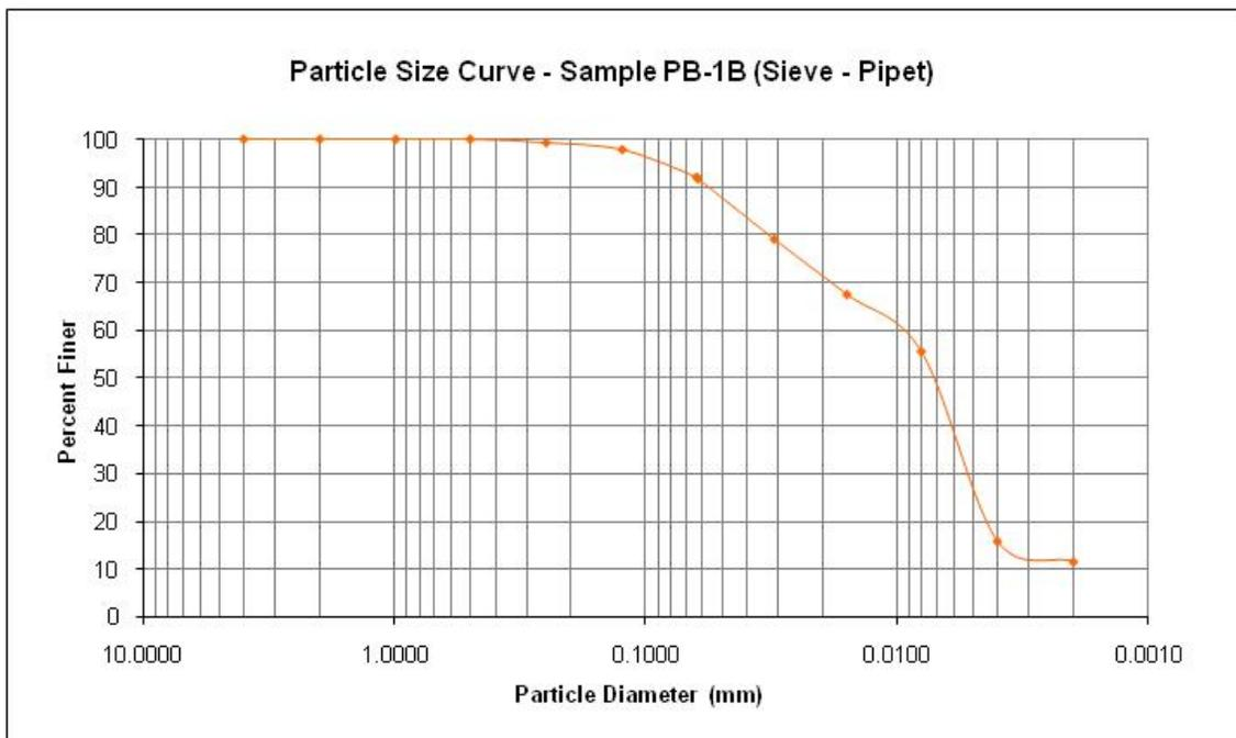
Figure 21 Gradation of PB-1B (Pipette)
