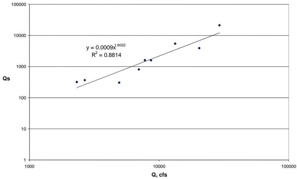
Figure 13 Sediment Rating Curve for the USGS Station 02489500
