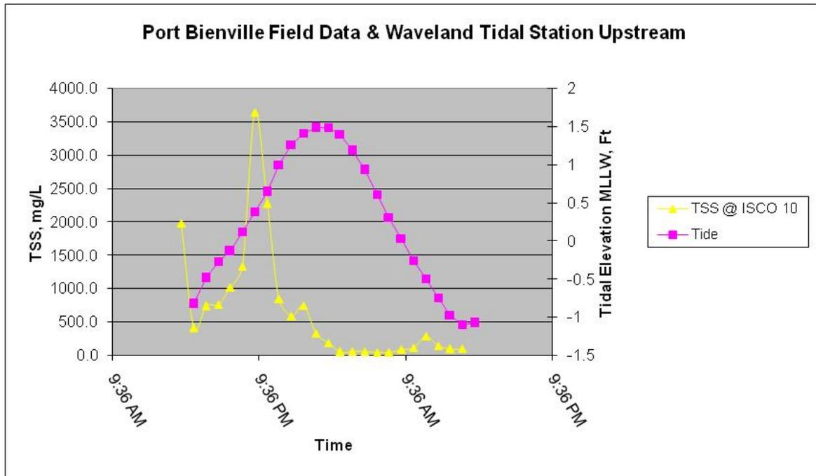
Figure 19 ISCO 10 Samples inside the Port
