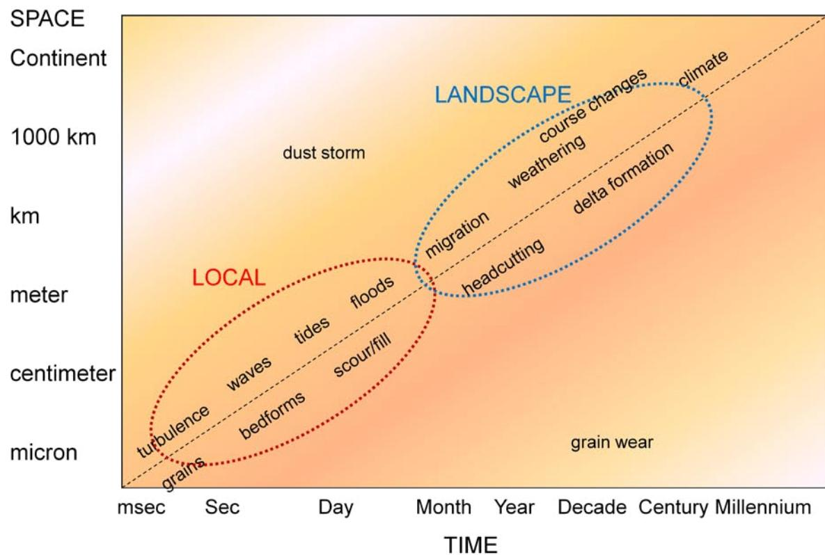
Figure 3-6. Comparable time and space scales for processes related to sediment transport.
