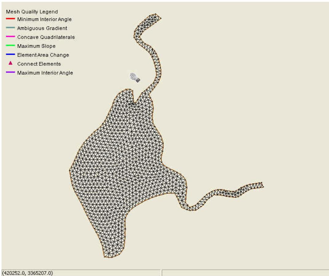
Figure 4-6. Computational mesh for a numerical model of water levels, flows, and constituent transport.
