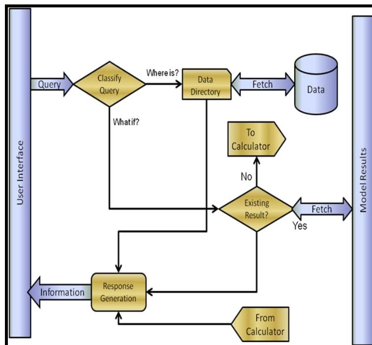
Figure 4-12a. Flow chart for Responder section of Inference Engine
