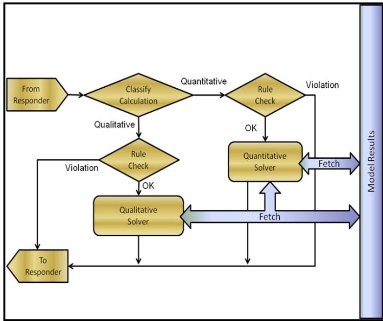
Figure 4-12b. Flow Chart for Calculator section of Inference Engine
