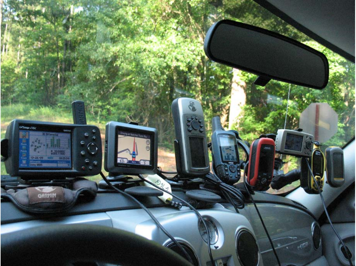
Figure 1. GPS receivers mounted and ready for testing conducted in five transportation settings at eight locations in seven major Mississippi cities.
