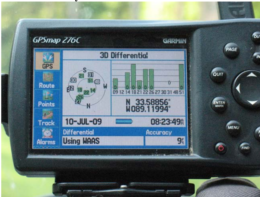
Figure 3. Garmin GPSmap 276C display. Notice the display size, WAAS enabling, and ~9 ft accuracy with seven satellites.
