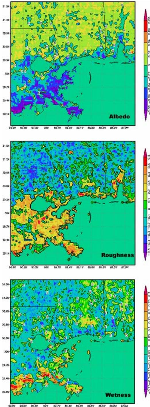
**Figure 3:** Differences between MODIS and USGS GLCC derived initial fields (MODIS - GLCC) of albedo (top), surface roughness (middle) and ground wetness (bottom) for the 3-km domain.
